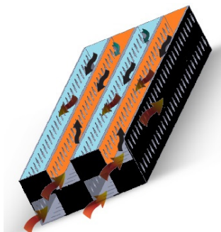
Figure 5. Cross-section view of a selective catalytic reduction type novel catalytic converter
