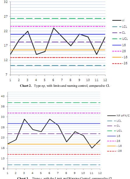
Chart 3. Ttype c, with the Limit and Warning Control, compared to CL
