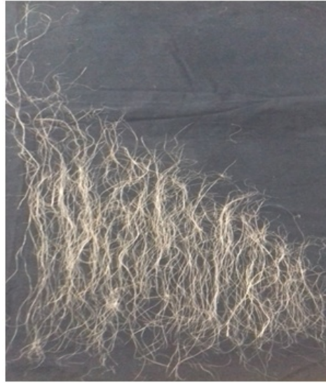
Figure 1. Fibers of finisher card sliver in decreasing order of length
