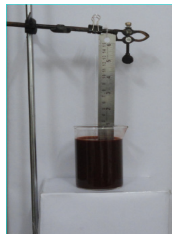
Figure 1. Wicking set-up for yarn
