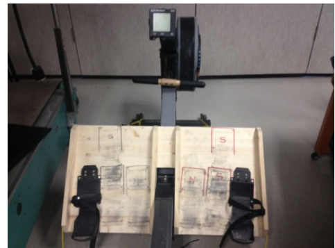
Figure 2. Foot-stop modification for a wide stance
