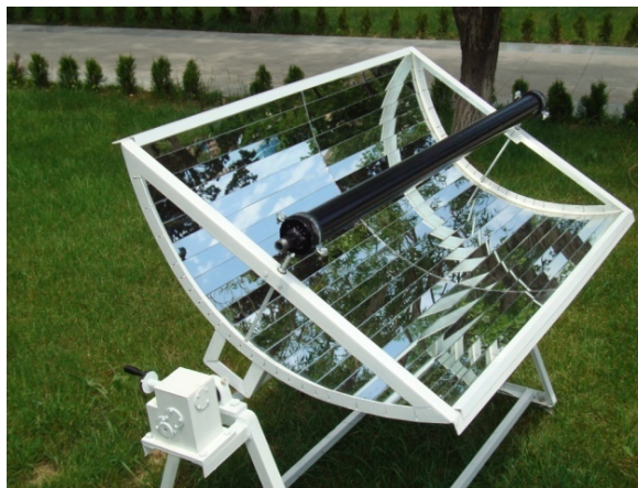
Figure 2. General view of the parabolic trough solar energy plant
