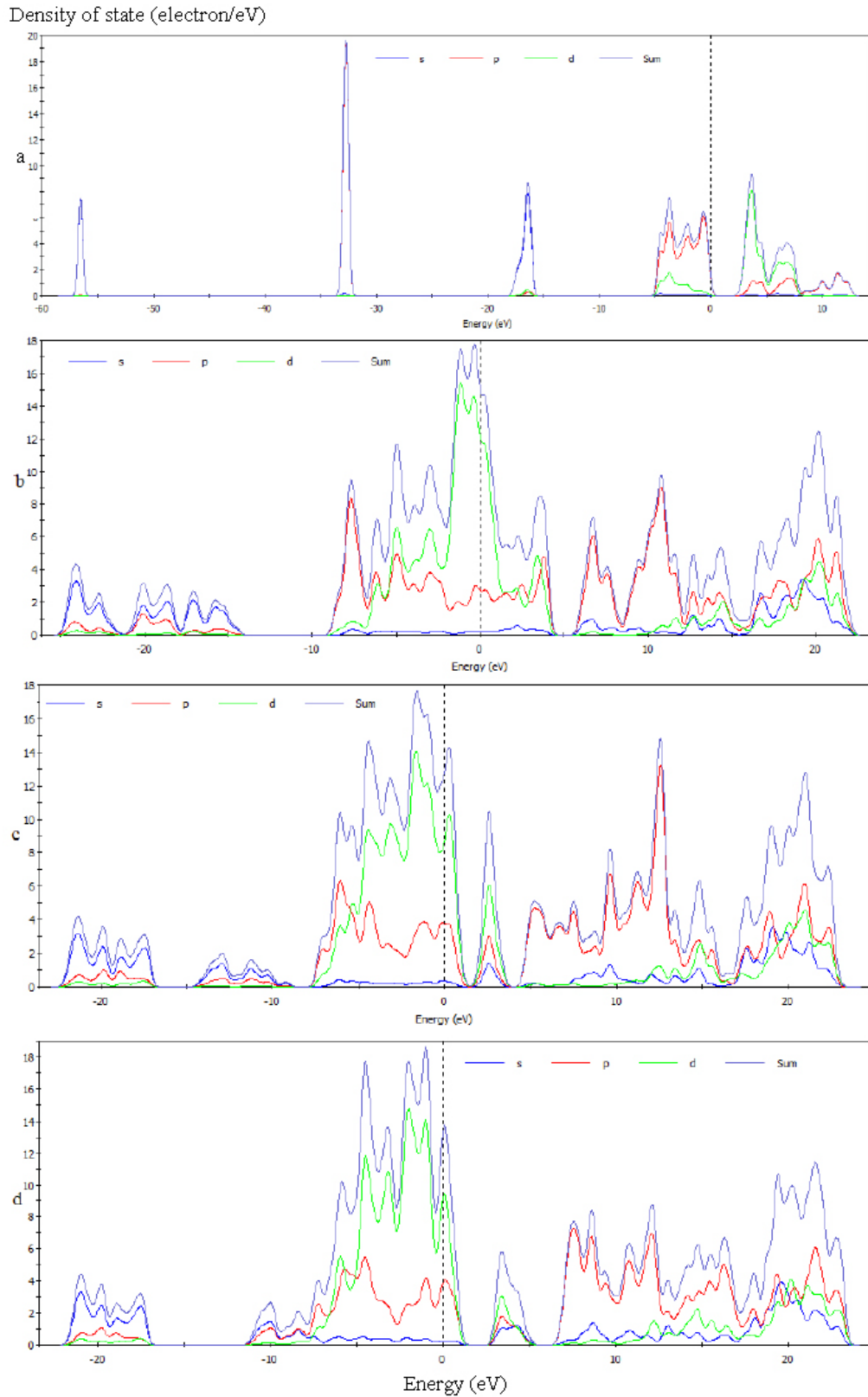
Figure 3. Density of states (DOS) of undoped TiO 2 (a) and TiO 2 doped with Co 15 % (b), 20 % (c), 25 % (d). The vertical dotted line is the Fermi energy level
