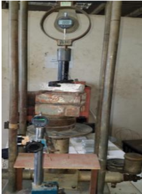
Figure 7. Flexural test apparatus
