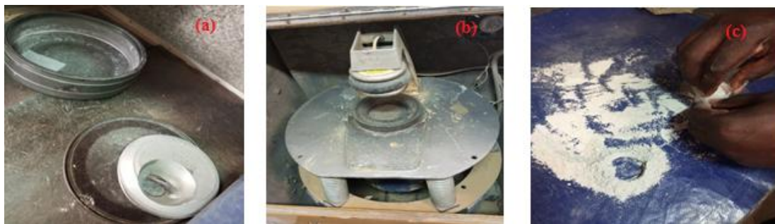
Figure 3. Spray equipment. (a) Tray, (b): Crusher, (c): Powder found after spraying
