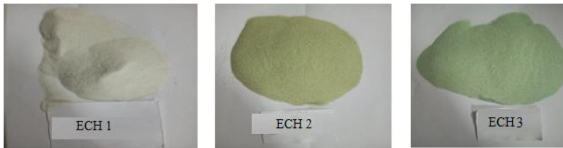
Figure 2. Crushed and sieved glass powder waste
