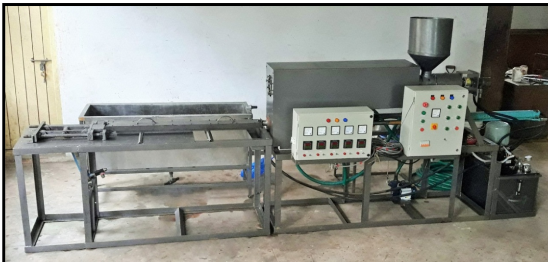
Figure 3. Photograph of the final assembled Two-stage Extruder-Injection molding machine
