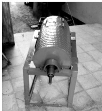
**Figure 1.** Cassava peeling machine with fixed outer peeling drum
