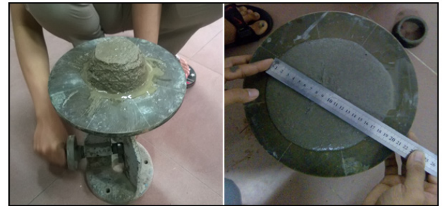
Figure 2. Measuring the workability of a sample
