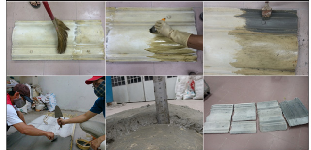
Figure 9. The process of fabricating the decorative panels
