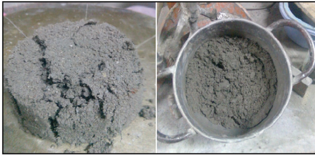
Figure 3. A sample with the low workability makes it hard to shape
