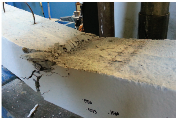
Figure 17. Concrete crushing due to static load
