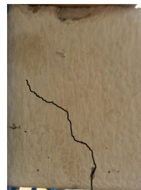
Figure 19. Crack initiation in prestressed beam, PC1, subject to impact
