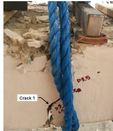
Figure 29. Failure of fiber-reinforced prestressed beam, FFH, subject to impact
