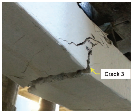
Figure 16. Beam failure due to static load
