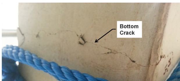
Figure 28. Tensile crack at the bottom of the fiber-reinforced prestressed beam, FFH, subject to impact
