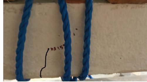
Figure 23. Crack initiation in the fiber-reinforced prestressed beam, UNH, subject to impact
