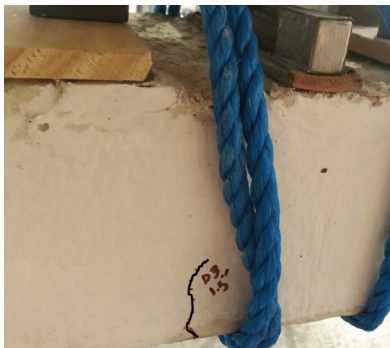
Figure 27. Crack initiation in the fiber-reinforced prestressed beam, FFH, subject to impact
