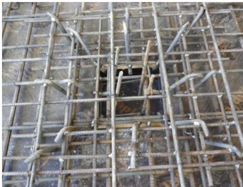
Figure 4. Reinforcement detail of specimen the third sample -PSW14-8
