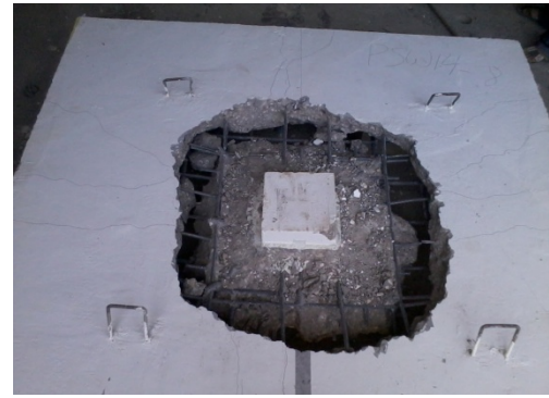
Figure 8. Failure mode of the 2mx2m PSW14-8 slab at 660 kN central load
