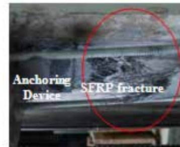
Figure 7. Fracture of SFRP (Type2)
