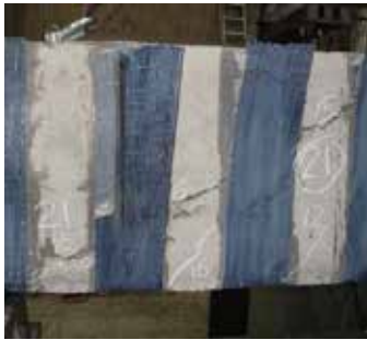
Figure 10. CFRP debonding
