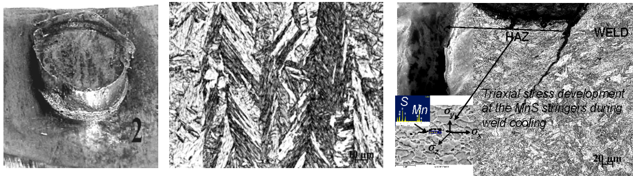
Figure 4. (a) Showing a representative photograph of pullout button failure, (b) showing OM micrograph of predominantly martensitic structure in weld zone (c) OM micrograph showing liquation crack in the fusion line[FEG-SEM magnified view in the top-left inset] along with HAZ crack at the Mn-S stringers[bottom-left inset] for annealing cycle 14-CR-1
