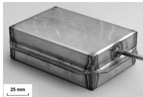
Figure 2. Example TIG welded stainless steel box prior to hot rolling[12]
