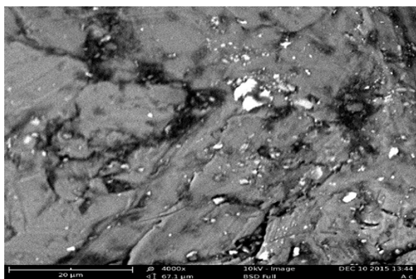
Plate 9. SEM photograph for Al- 4%wtCu (X4000)
