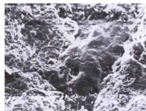
Cliché V.3. X100Cr12 steel V notched specimen, at room temperature, N=67300 cycles
