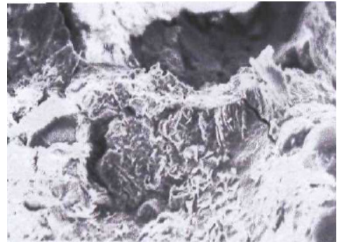
Cliché V.9. XC18 steel smooth specimen, at room temperature N= 719300 cycles
