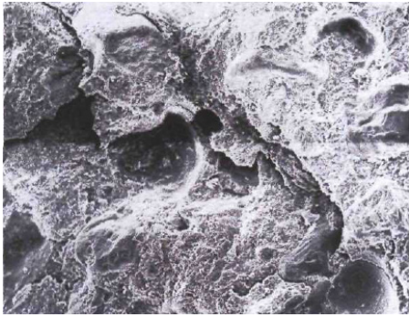
Cliché V.5. X100Cr12 steel smooth specimen at T= 200^{\circ}\text{C} , N= 745651 cycles
