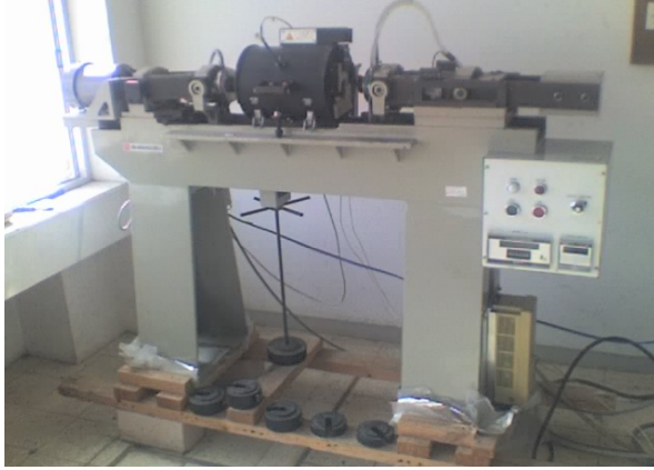
Figure 5. Rotary bending machine H7 (SHIMADZU)
