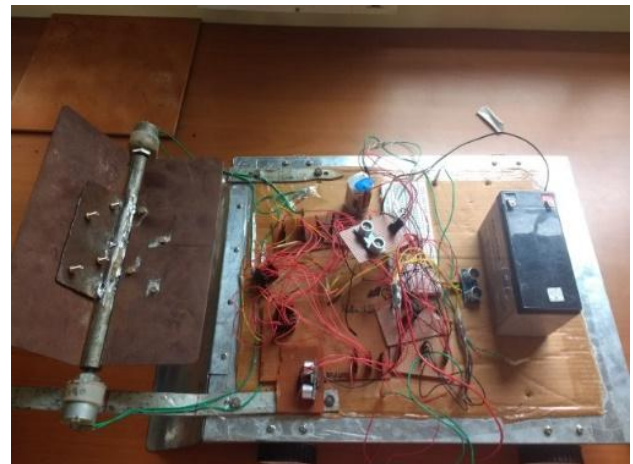
Figure 5.1. Skeleton of the bot from top view
