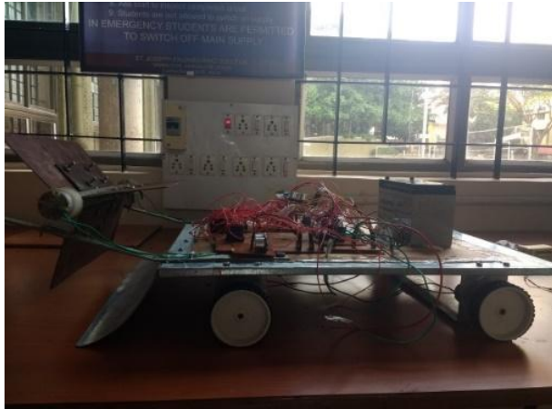
Figure 5.2. Skeleton of the bot from side view
