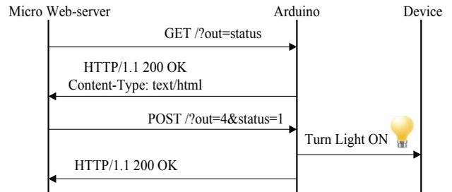
Figure 4. Messages between Arduino and micro Web-server
