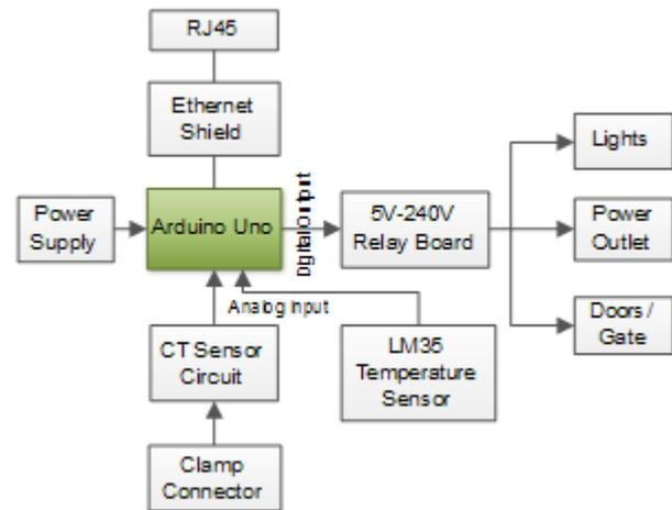
Figure 6. Hardware architecture and implementation
