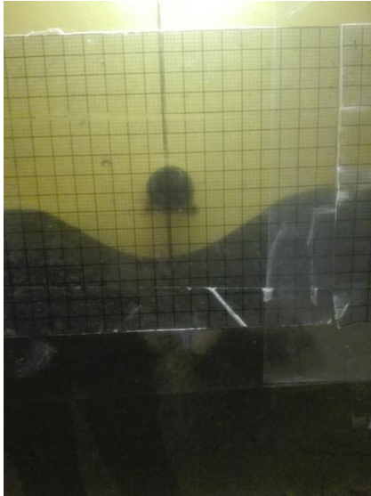
Figure 3. Checkered plates used for drawing the scour profile
