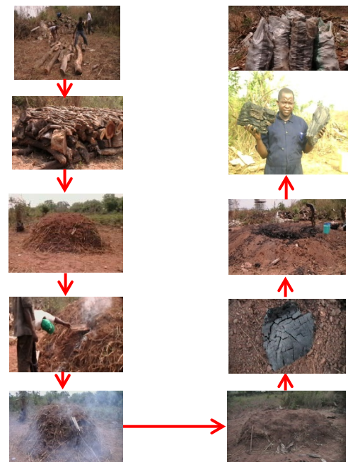
Plate 4. Picture Chart of Pyrolysis Processes using Earth Mound Method
