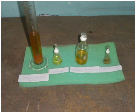
Figure 2. Plastroleum, Naptha, Middle Distillate and Heavy Cut oil Derived from Hydropyrolysis process
