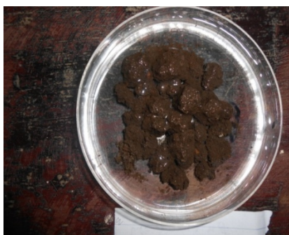
Slaking process of E. Leptosol and E. Vertisol after 30 mins
