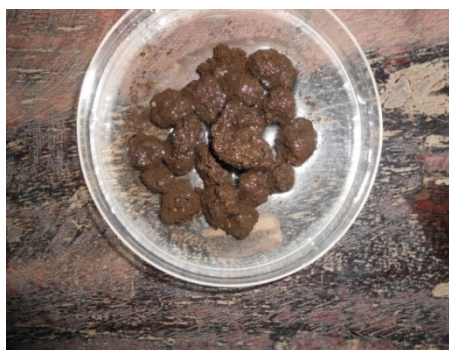
Slaking process of E. Leptosol and E. Vertisol after 20 mins
