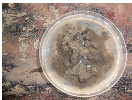
Slaking process of E. Leptosol and E. Vertisol after 30 mins
