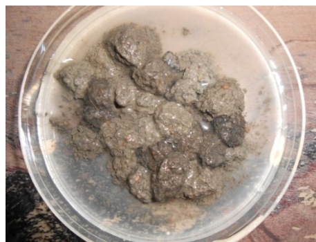
Slaking process of E. Leptosol and E. Vertisol after 20 mins
