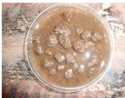
Slaking process of E. Leptosol and E. Vertisol after 40 minutes
