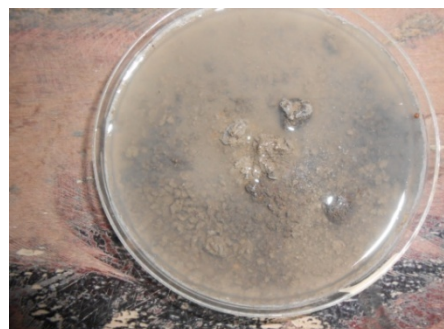
Slaking process of E. Leptosol and E. Vertisol after 24 hours
