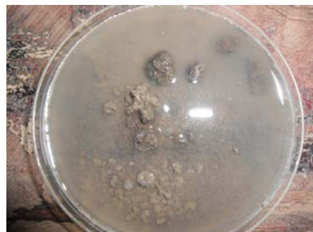
Slaking process of E. Leptosol and E. Vertisol after 40 minutes
