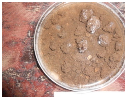
Slaking process of E. Leptosol and E. Vertisol after 24 hours
