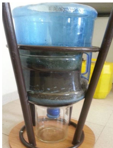
Figure 2. The home-made filter showing the process of filtration
