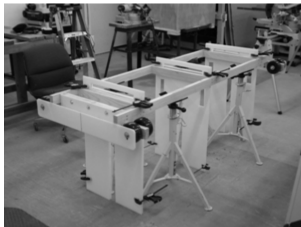
Figure 2. The Mark II prototype tested guide strips (rectangular high density polyethylene (HDPE) pieces bolted to each end), polyurethane wheels (5-in diameter x 2-in width), and panel holding devices (large, slotted panels of HDPE)
