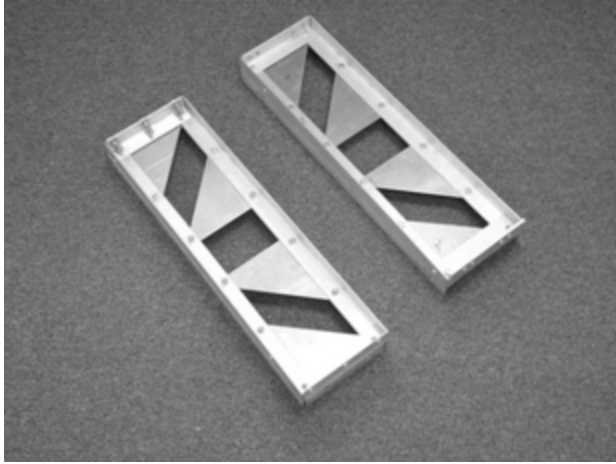
Figure 4. Supports designed for the push bar on the Mark III. The supports were comprised of extruded aluminum angle and 0.125 in thick aluminum Isosceles triangles. These supports were also used to reinforce the draw works on the Mark IV prototype. The design shown in this figure is complex and assembly is time consuming. The authors suggest that individual builders substitute a simpler design of their choice
