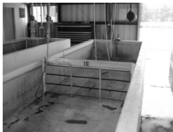
Figure 1. A grading panel designed for use in a rectangular concrete holding vat. Uniformly spaced rods prevent golden shiners Notemigonus crysoleucas having cross-section greater than 16/64 in from swimming through. Flexible strips attached to each end prevent fish from swimming around the panel. Workers use the ropes to pull the panel through a vat containing up to 400 lb of fish
