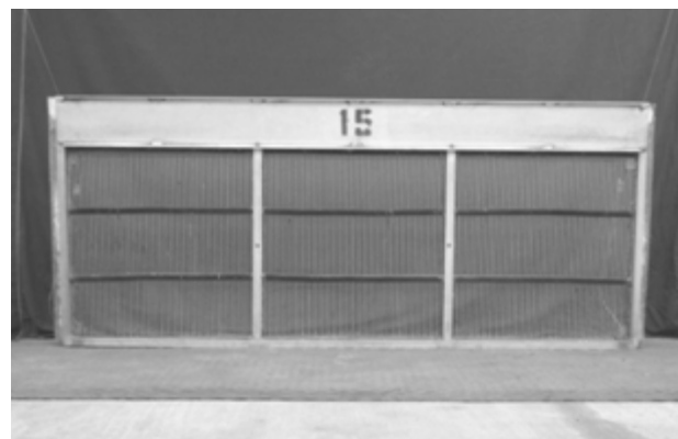
Figure 1. A number 15 grader of the type used to sort golden shiners into size-weight classes. The inch-pound system is used by U.S. bait fish farmers, and grader spacing is indicated in 64th inch increments. In a 15 grader, aluminum rods having diameter of 0.1875 inch are set on 0.4219 inch centers to provide a 15/64 (0.2344) inch space between adjacent rods. SI units: In a 5.96 mm grader, aluminum rods having diameter of 4.76 mm are set on 10.72 mm centers to provide a 5.96 mm space between adjacent rods
