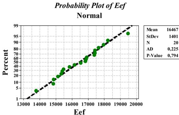
Figure 6. Normal probability plot for the modulus of elasticity  $E_{ef}$
