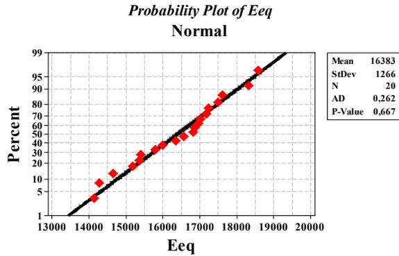
Figure 5. Normal probability plot for the modulus of elasticity  $E_{eq}$
