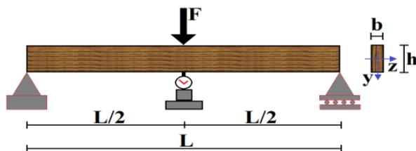
Figure 3. Static three-point bending tests[5]
