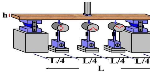
Figure 4. Alternative test to determine the effective modulus of elasticity
