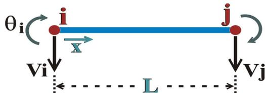
Figure 5. Finite-element degrees of freedom
