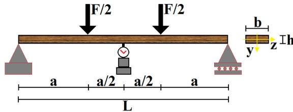
Figure 2. Four-point static bending[4]
