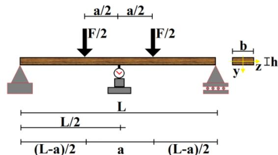
Figure 1. Static four-points bending tests[3]
