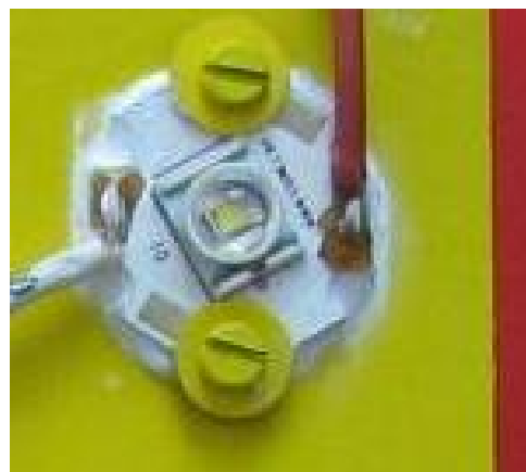
Figure 1. XLamp LED (XR-E) mounted on MCPCB
