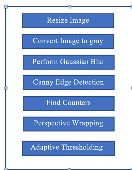
Figure 3. Steps for scanning the image
