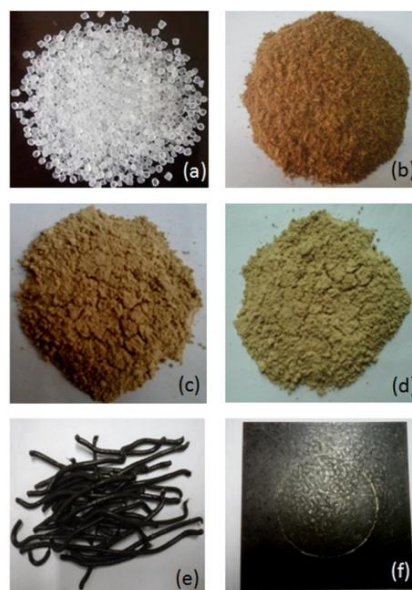
Figure 1. (a) Commercial PP pellets, (b) Rice husk, (c) Untreated rice husk, (d) Treated rice husk, (e) Extruded rice husk/PP samples, and (f) Fabricated composite sample
