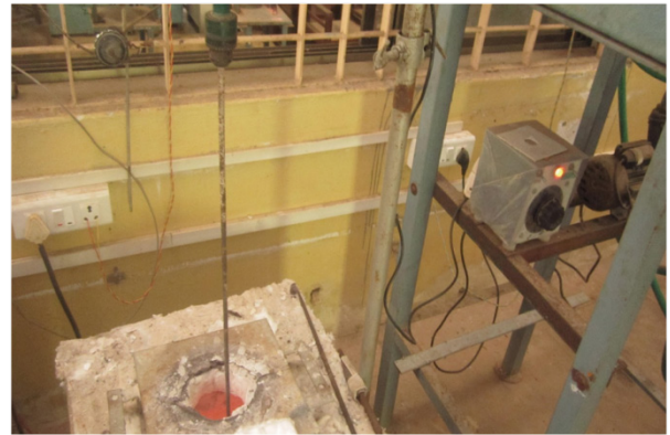
Figure 1. Experimental setup for stir casting Al 6061-TiB 2 composite
