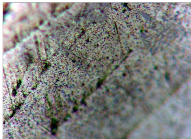
Figure 4a). Micrograph of Al 6061 alloy, as cast (100X)
