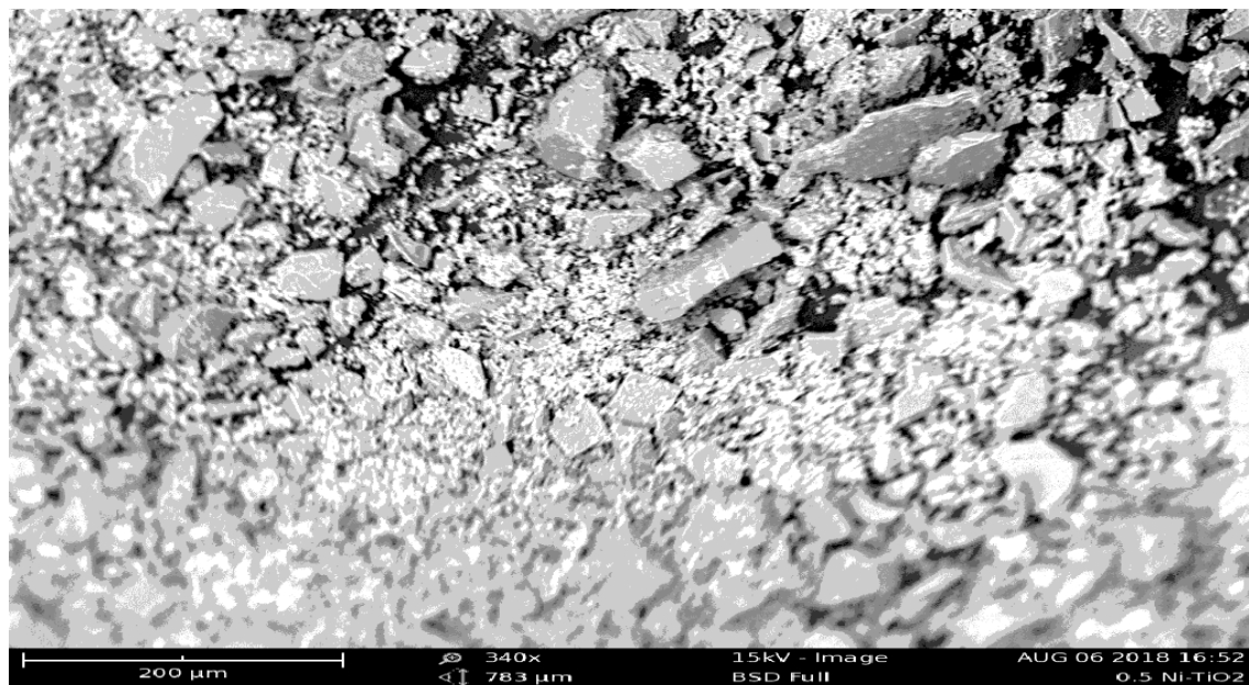
Figure 1. Scan electron microscopy of 0.5% Ni-TiO 2
