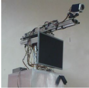
Figure 2. Flexible robotic arm assembly on mobile robotic platform.
