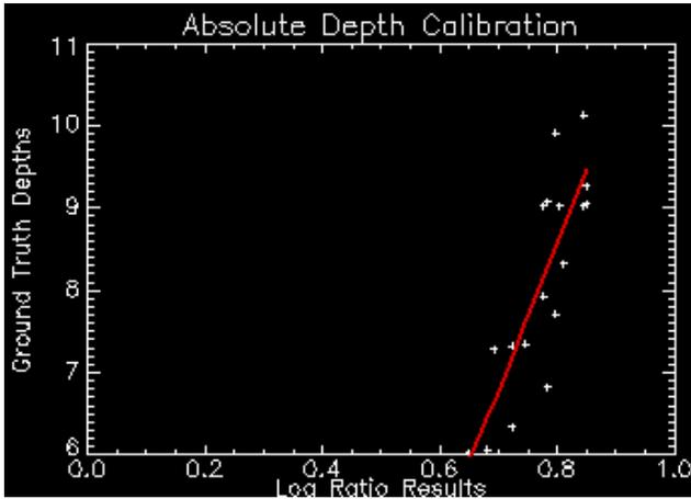
Figure 6. Imagery Absolute Depth Calibration Using Linear Method
