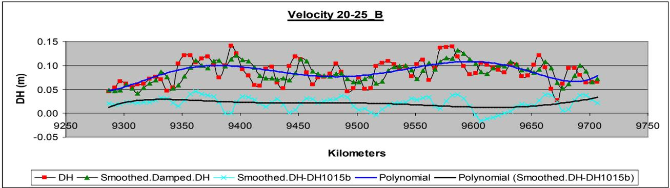
**Figure 9.** Height differences per kilometer, their correspondent smoothed height differences and residuals for velocity passing 20-25B (km/h) and reduced velocity passing 20-25B (km/h) to 10-15B (km/h)
