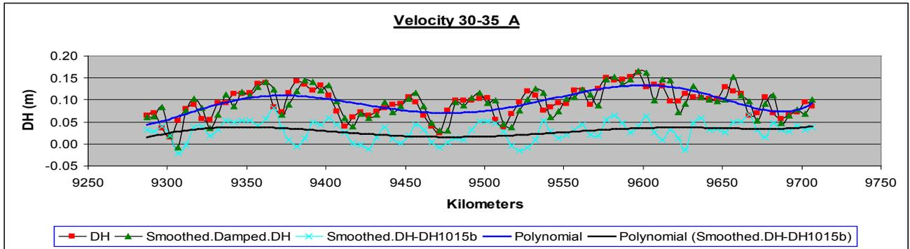
**Figure 10.** Height differences per kilometre, their correspondent smoothed height differences and residuals for velocity passing 30-35A (km/h) and reduced velocity passing 30-35A (km/h) to 10-15B (km/h)
