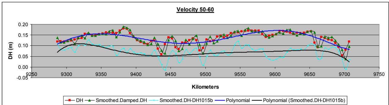
**Figure 12.** Height differences per kilometre, their correspondent smoothed height differences and residuals for velocity passing 50-60 (km/h) and reduced velocity passing 50-60 (km/h) to 10-15B (km/h)
