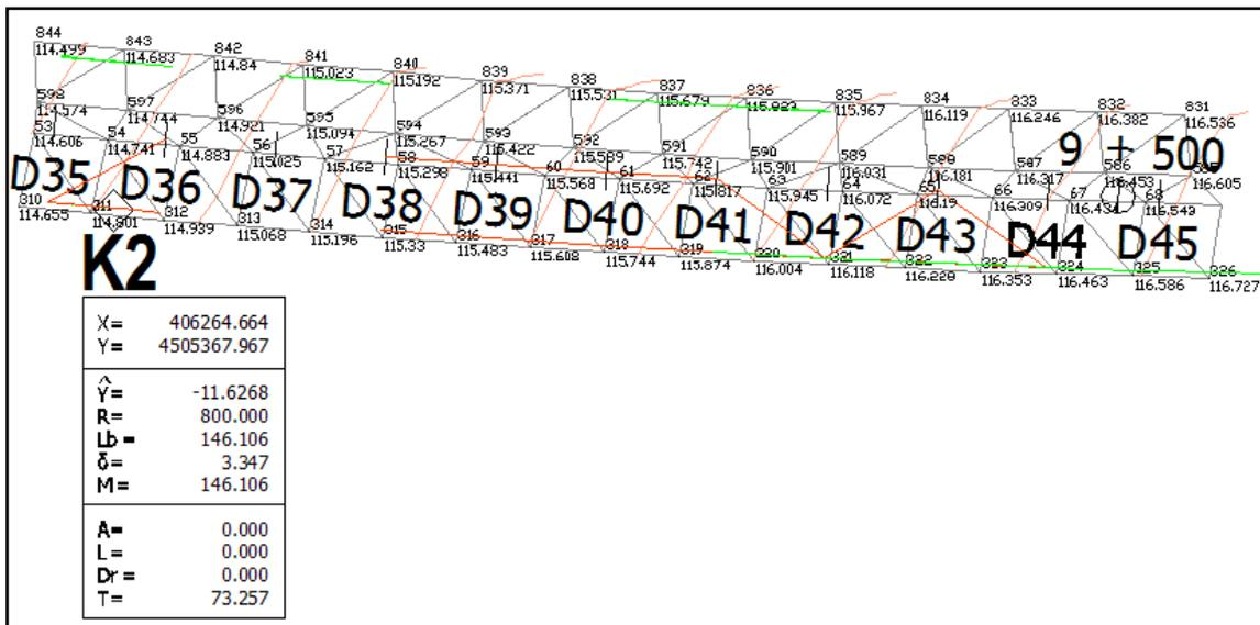
Figure 3. Detail of the reconstructed road horizontal plan, DPSM by velocity 20-25 km/h, passing B
