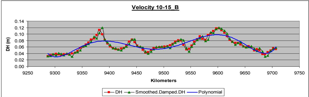
**Figure 6.** Height differences per kilometre, their correspondent smoothed height differences and residuals for velocity passing 10-15B (km/h), which was used as zero-measurement
