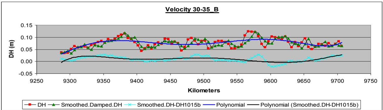
**Figure 11.** Height differences per kilometre, their correspondent smoothed height differences and residuals for velocity passing 30-35B (km/h) and reduced velocity passing 30-35B (km/h) to 10-15B (km/h)
