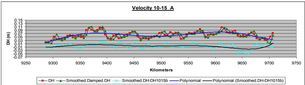
**Figure 7.** Height differences per kilometre, their correspondent smoothed height differences and residuals for velocity passing 10-15A (km/h) and reduced velocity passing 10-15A (km/h) to 10-15B (km/h)
