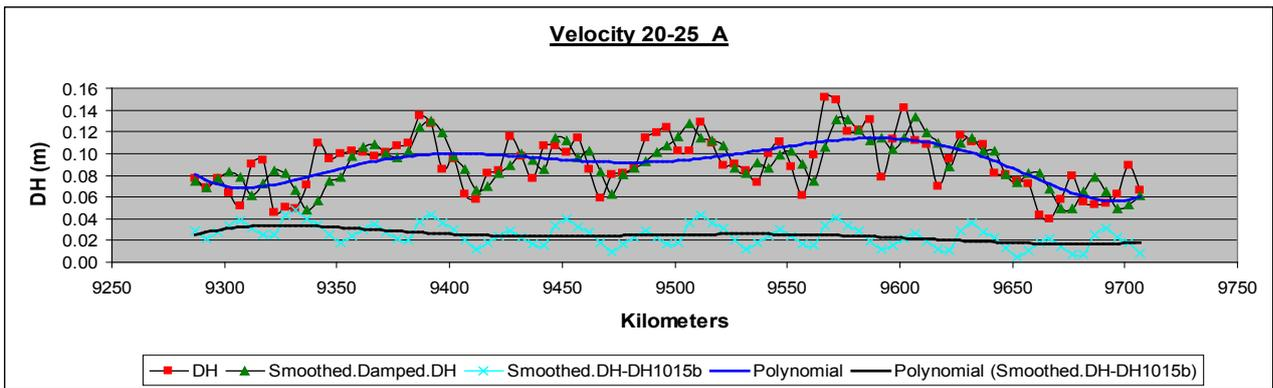
**Figure 8.** Height differences per kilometre, their correspondent smoothed height differences and residuals for velocity passing 20-25A (km/h) and reduced velocity passing 20-25A (km/h) to 10-15B (km/h)
