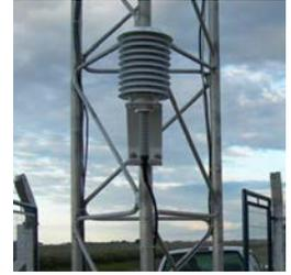
**Figure 3.** a) Tower, surrounded by fence, the dog house was protecting the spare battery, b) triaxial anemometer and carbon dioxide and vapor analyzer on the top, while net radiometer is below, and c) sensor of temperature and humidity
