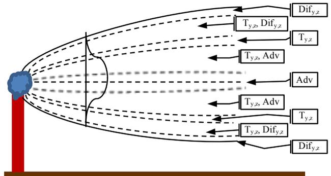
**Figure 1.** Schematic drawing of the pollutant plume, showing regions of dominance of the terms in equation (3)
