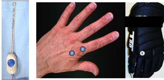
Figure 3. Three thin film sensors were used; one on the outside of the glove over the distal end of the second metacarpal (1) and two on the inside the glove, one (2) at the same location as outside sensor and the other (3) over the proximal phalanx
