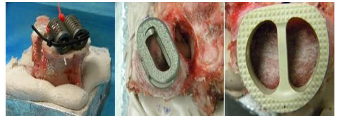
Figure 1. Intervertebral implants tested. A) Threaded-Titanium (paired), B) Oval-Titanium, C) PEEK
