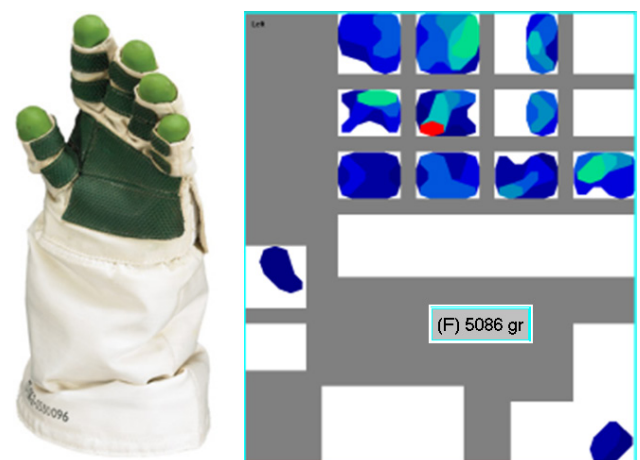
Figure 7. Pressure distribution in a power grip movement wearing the EVA glove
