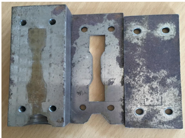
Figure 2. Die Cavity
