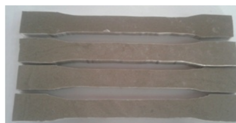
Figure 3. Tensile Test Specimens
