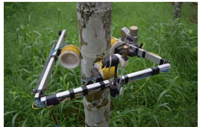
Figure 2. Arecanut climbing and spraying machine
