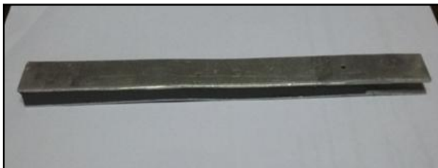
Figure 3. Photograph of MRE sandwich beam
