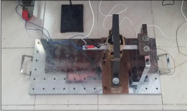
Figure 5. Experimental setup for vibration analysis of the MRE sandwich beam
