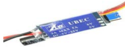
Figure 2. Universal Battery Eliminating Circuit
