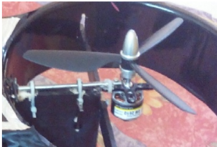
Figure 4. Tilt motor mechanism
