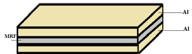
Figure 1. MR Fluid sandwich beam
