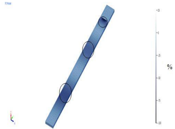
Figure 8. The change in young's modulus in the steel plate after updating the calibrated finite element model with the obtained damaged data
