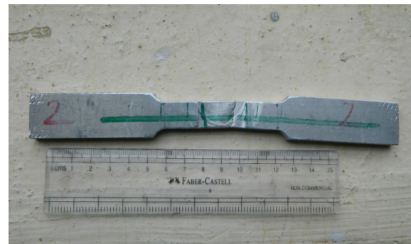
Figure 4. Specimen as subjected to tensile test
