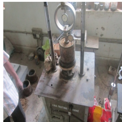
Figure 4h. Sample tested with CBR machine
